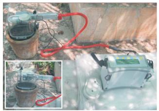
Figure 2: Measurement of media respiration rate with LC pro+instrument (inset: soil chamber)
